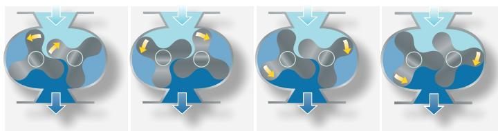
**4 → 1 Suction.** Air enters the compression chamber. The air volume remains constant while the lobe rotors turn.
