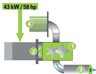
In the ZS screw blower, the internal air flow path is optimized to reduce pressure drops and air turbulence.
