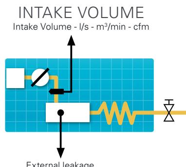
Inlet flow referred to blower element inlet conditions. Seal leakages and inlet losses should not deprive you of the air you paid for.
